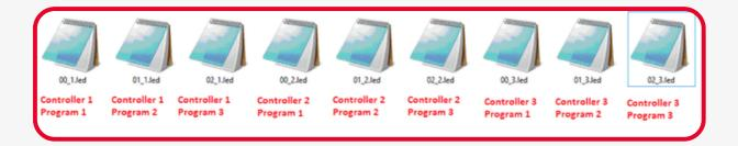
If you are using multiple controllers networked together, you only need a single SD card inserted into the first controller in the network. You can place each controller's programs inside that SD card.
