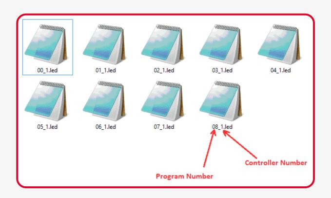
If you are using a single controller or multiple controllers without networking them (in this case, every controller has an individual SD card), the file placement for each controller SD card would be like this: the first two digits stand for program number (00 to 16). Since we use a single SD card for each controller, the last digit is always "1".
